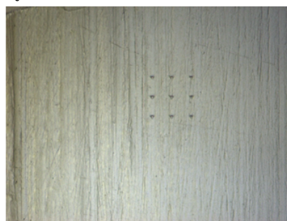
Fig.5 PMMA specimen tested by indentation
